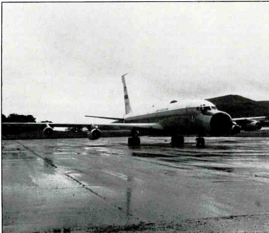
One of the 4950th Test Wing's ARIA aircraft sitting on the runway at Easter Island. This C-18 and an EC-135, both from the 4950th TW, Wright-Patterson AFB, Ohio, were used by ARIA to provide telemetry checks of a DOD satellite released by the space shuttle Atlantis. (U.S. Air Force by SSgt. Michael Riley).
