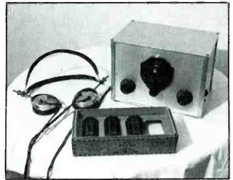
David Ivarson's resurrected 2-tube regen receiver. The Bud plug-in coils are still in their original 1940's box.
